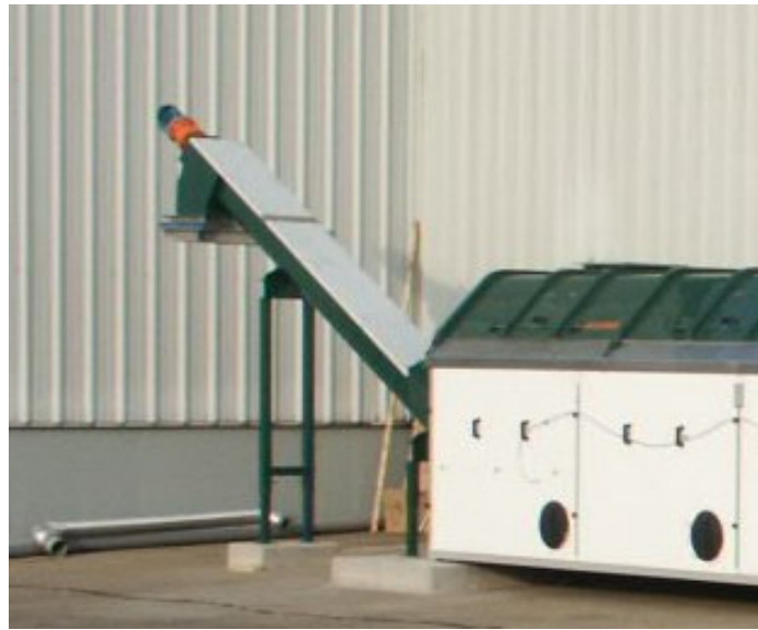
Incline discharge auger installed on smaller HotRot 1811 composting unit
